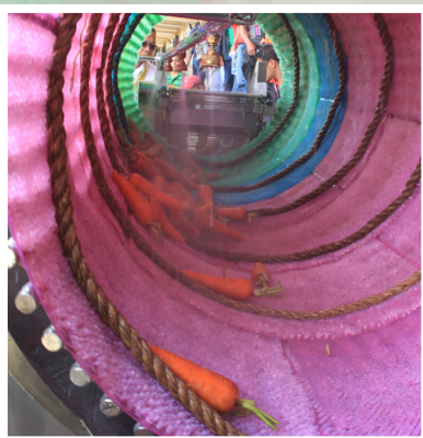
The actual operation of rootcrop washer as the carrots move forward inside the rotating tumbler with high-pressure water continuously sprayed.
